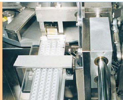
Feeding of filled diagnostic capsules into an assembly machine
