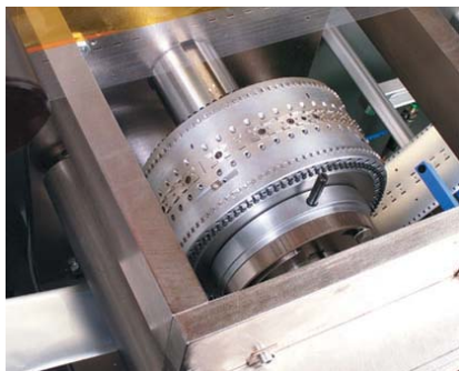
Precise die-cuts by means of servo-controlled tools
