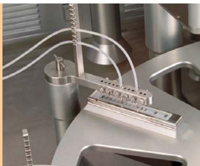
Dosing liquid with peristaltic pumps
