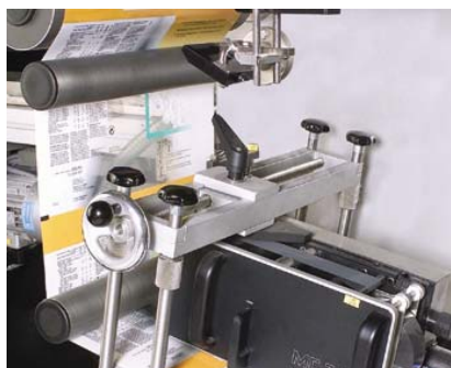
Coding with hotleaf printer, with subsequent print mark check
