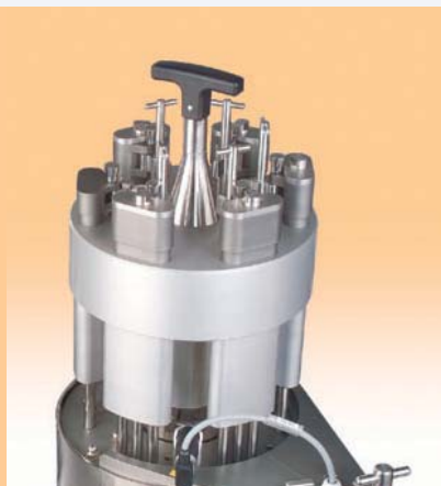
Tamping pin system with compaction
