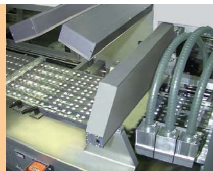
Camera control with the subsequent extraction of product dust
