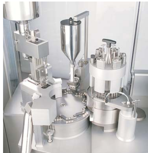
The basis for a reliable weighing process – the turret of the Modu-C
