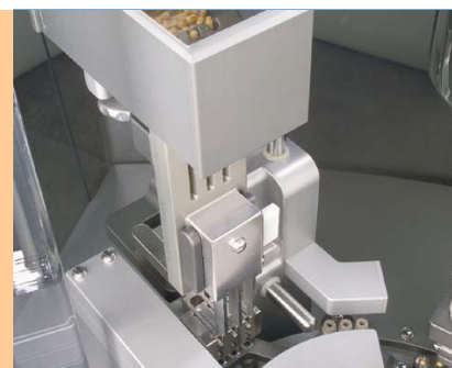
Inserting of empty capsules into the rotary turret
