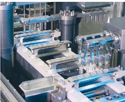
Assembly line for completion of the injector components
