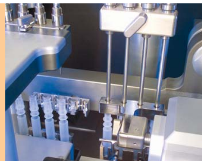
Dosing of the active substance into the previously turned injectors
