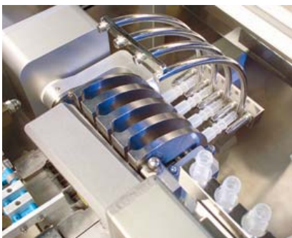
Introduction of the injector bodies, assembly and filling
