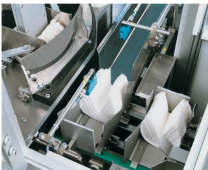
Two feeds for normal and folded (boutique) tissues for the highest degree of efficiency
