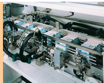
Gluing and subsequent closing of cartons
