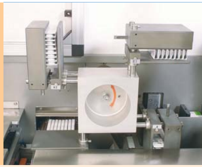
Turning wheel for turning the packages to the correct position before cartoning
