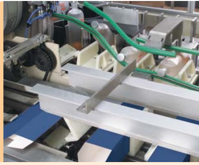
Feeding, tilting and insertion of bottles into the prismatic chain
