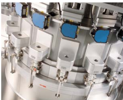
Conveyance of the inhalers in the turntable to be inspected
