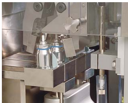
Pressing of the cartridges into the bottom side of the counter
