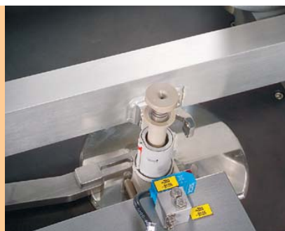
The laser controls the spray jet within a defined tolerance range
