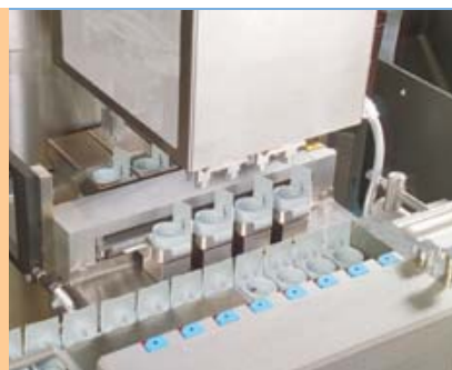
4-fold transfer of the bottom parts into the turntable
