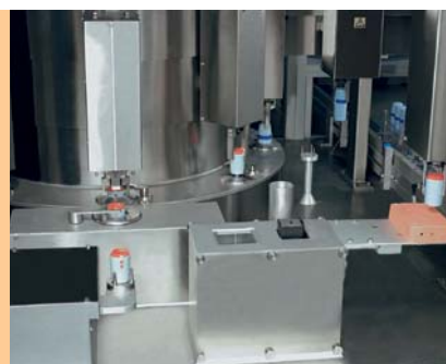
Powder filling and compaction in the powder chamber
