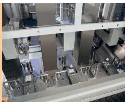
Feeding and orientation of the turntables for final assembly of the inhaler with a functional test
