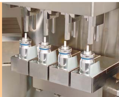
Checking of the assembled products to the correct pressing-in dimension
