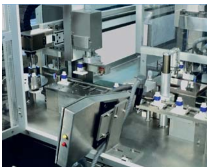
Tara - gross weighing with laser coding and fail-part removal
