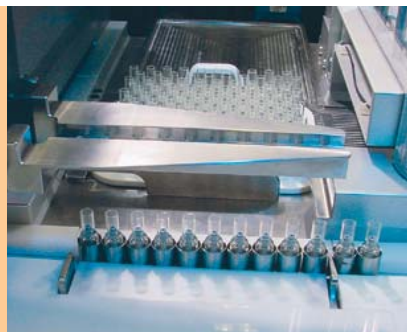
Unloading of the ready assembled products from the puck conveying system
