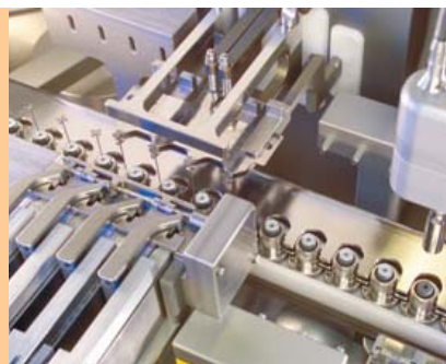
Insertion of the needles into the stoppers and discs
