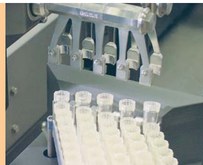
Transfer of the injector components by means of grippers
