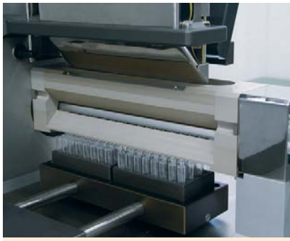
The laboratory machine for the dosing of micro-quantities of powder with extremely high precision
