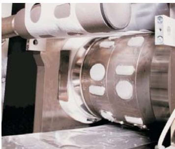
Die-cutting and introduction of fabric pads into the cold-formed foil
