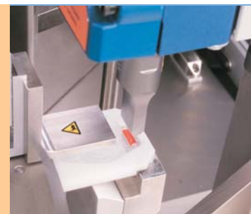
Ultrasonic welding of code strip in syringe gripper
