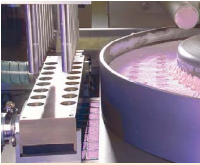
Filling the tabs with powder using the dosator
