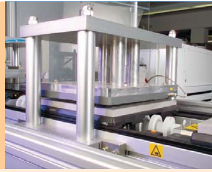
Hot sealing of the lidding foil onto the molded film pack
